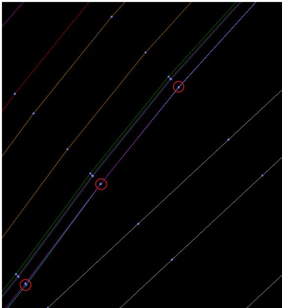
**Note:** to view the nodes of the line marking in the plan view like the image to the left, click the
