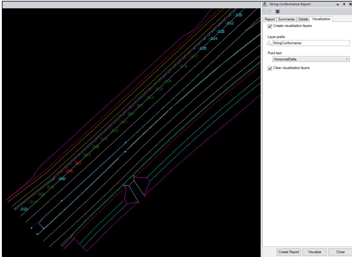
**Green** means the node is within tolerance. **Cyan** means the node is either to the left of the design or below it. **Red** means the node is either to the right of design or above it.
